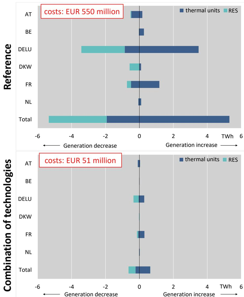
Figure 3-9: Comparison of redispatch volumes and related costs when combining the three technologies with the reference scenario
