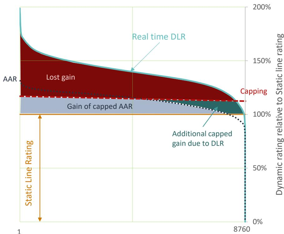
Figure 2-1: Illustration of capping mechanism
