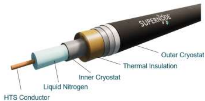
Figure 3. Structure of an HTS DC cable.
